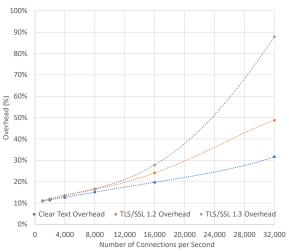
In the figure on the left, we see how content transferred declines when the number of connections increases. Since the overhead is constant for each connection, increasing the connections per second means less bandwidth for content.
